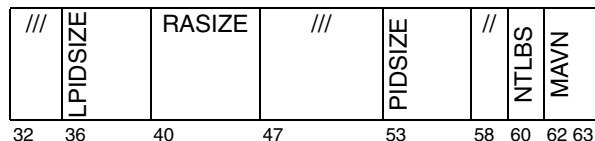
Figure 28. MMU Configuration Register [MAV=1.0]
